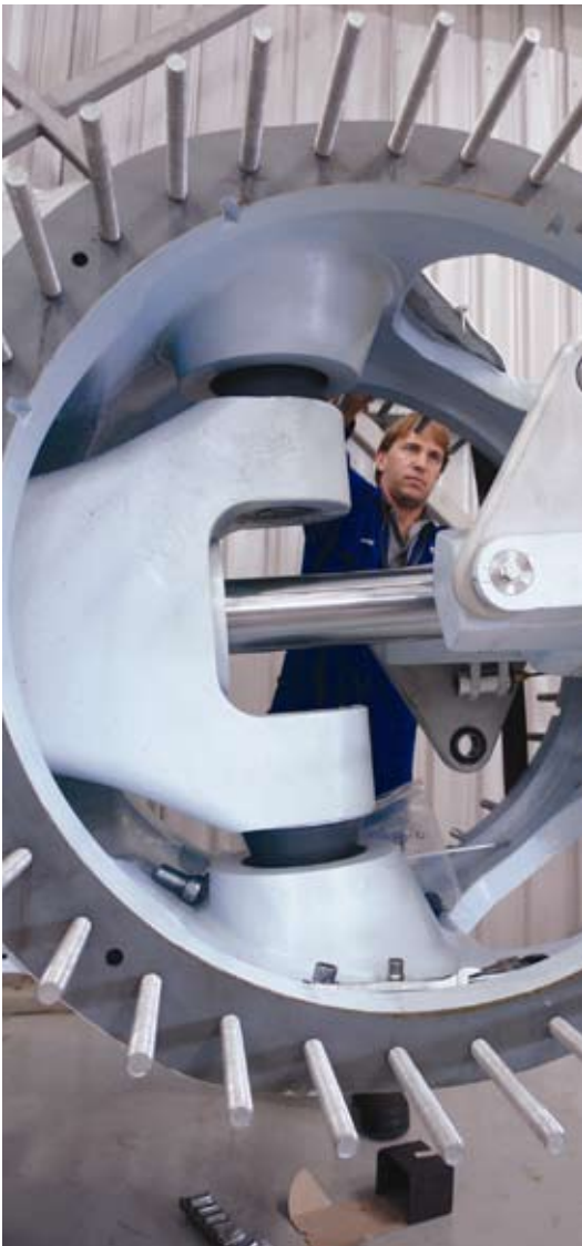
An employee of HERA member Windflow Technology working on the hub of the Windflow 500 turbine, designed and assembled in Christchurch. The wind turbine has a 90% kiwi content with parts sourced from all over New Zealand.
