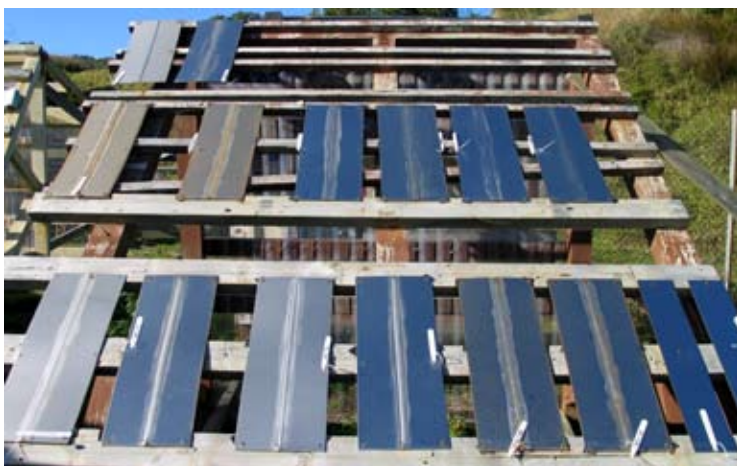
Performance evaluation of alternative stainless steel grades - testing of welded samples at Muriwai Beach testing site
