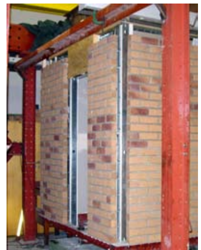
Full-scale light steel frame specimen prior to shaking table tests at the University of Melbourne
