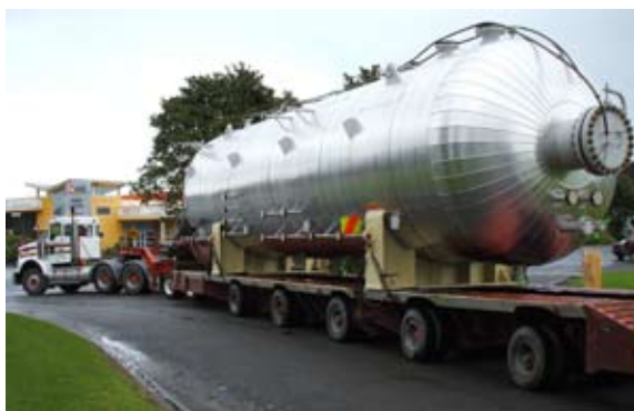
Duplex HP gas separator for Kupe gas field by HERA member Fitzroy Engineering
