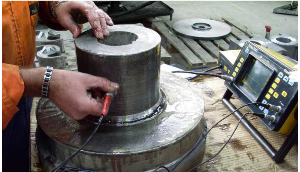
Non-destructive testing by HERA member Southern QA for wind power project components (courtesy of Wade Engineering)
