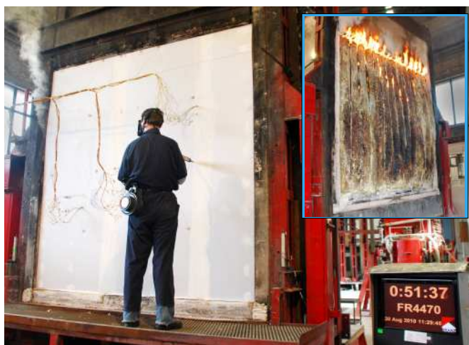
CSA panel undergoing a loaded fire test to EN 1365-1: 1999 at BRANZ. The panel achieved a 53 minute fire rating under a 75kN/m load
