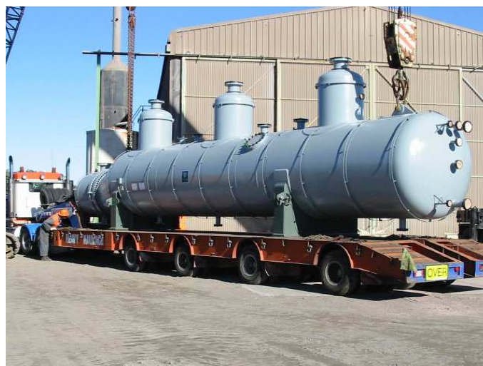
Geothermal heat exchanger loadout (photo courtesy of HERA member Fitzroy Engineering)
