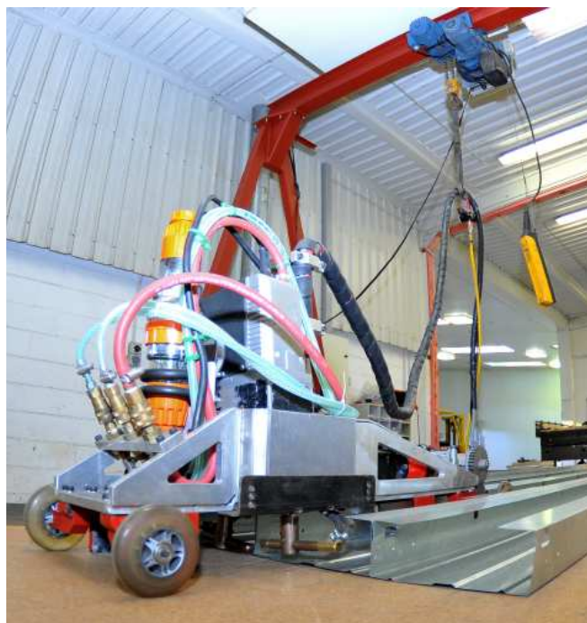
NZ Welding Centre-developed automatic resistance spot welding system in operation at the CSA pilot plant
