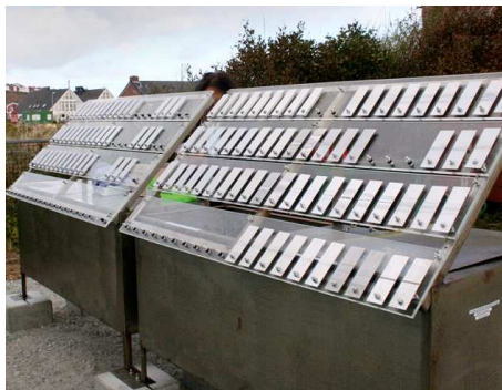
A set of New Zealand stainless steel samples exposed on North Sea island of Helgoland, Germany
