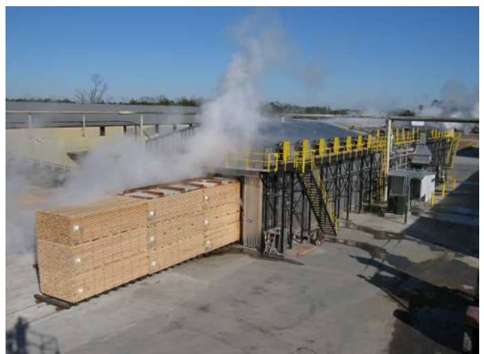
Metal engineering supporting sustainable timber as demonstrated by HERA member Windsor Engineering who produced the world's first steam-heated continuous drying kiln (CDK) early this year
