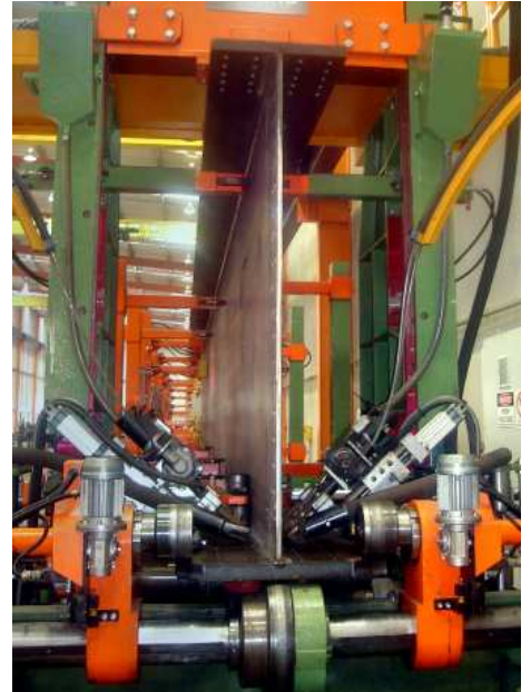
The steel fabrication industry has invested heavily in more productive plant over recent years. This photo is from the new Welded Beam Line installed at HERA member Dixon and Haddon. The product fabricated here are the Kopu bridge girders.
