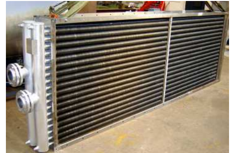
Hamilton-based HERA member Advance Boiler Services Ltd tackles import replacement work with their fabrication of an oil heater for use in the pulp processing industry.
