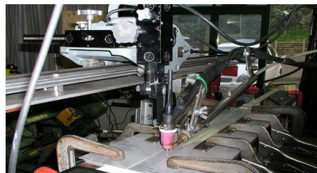
TIG welding of stainless steel samples used in corrosion test
