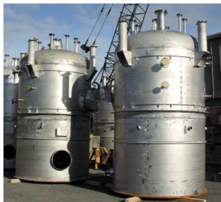
Super Duplex Salt Dissolver Vessels at HERA member Fitzroy Engineering fabrication yard bound for the Gorgon LNG project West Australia
