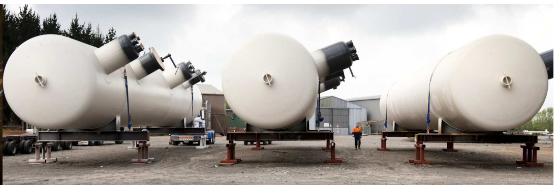
HERA member Tenix New Zealand was awarded a contract to design, fabricate and deliver four mounded pressure vessel 'bullets' for Transfield Worley Services Ltd. The pressure vessels are for a new Liquefied Petroleum Gas (LPG) Recovery, Storage and Load-Out project at Todd Energy's McKee Oilfield Production site in Taranaki.
