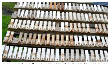
Exposure test on different grades of stainless steel at Muruwai beach
