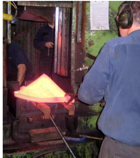
Hot forming of martensitic stainless hydro turbine runner blades on 1000kg drophammer by HERA member S.A.F.E. Ltd
