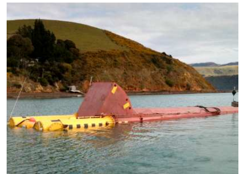
WET-NZ's half-scale wave energy device fabricated by Stark Brothers in Lyttelton being deployed for trials
