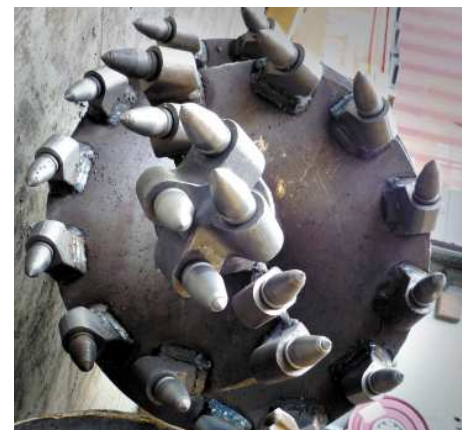
1-tonne auger with 1,500mm diameter fabricated by HERA member Parfoot Engineering used in the Victoria Park tunnel project
