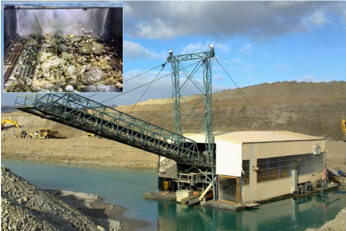
The L&MM plant is the largest, and arguably the most innovative, alluvial gold mining plant recently commissioned in NZ. It uses a feeder and horizontal scalping screen, followed by state-of-the-art jigs and concentrators to recover the alluvial gold. The re-build and commissioning of this floating plant provided significant heavy engineering work for several South Island engineering businesses. Inset: HERA member Niemac Industrial fabricated the primary scalping screen plasma cut from AR plate
