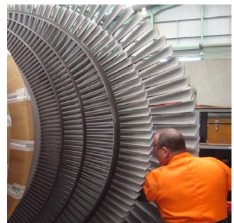
Geothermal turbine repair is routine work for HERA member Allied Industrial Engineering with an end-to-end process that includes repairs using specialist welding equipment and large machine tools and post-repair NDT inspection
