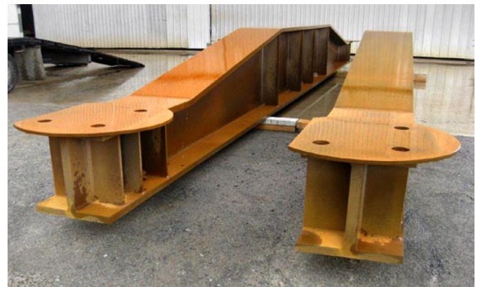
Aspects of weathering steel ballast deck railway bridges being fabricated at HERA member Culham Engineering in Whangarei. The first bridges go into service on 1st September.
